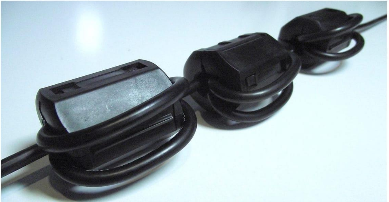
A run of RG58 coax on its way to a transceiver, via 3 large clamps, with 3 turns per clamp
