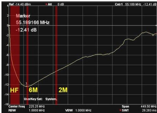
Using one Q2 ferrite clamp, looped twice
