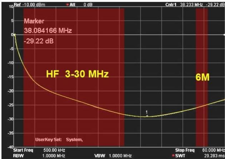
Using one Q2 ferrite clamp, looped five times
