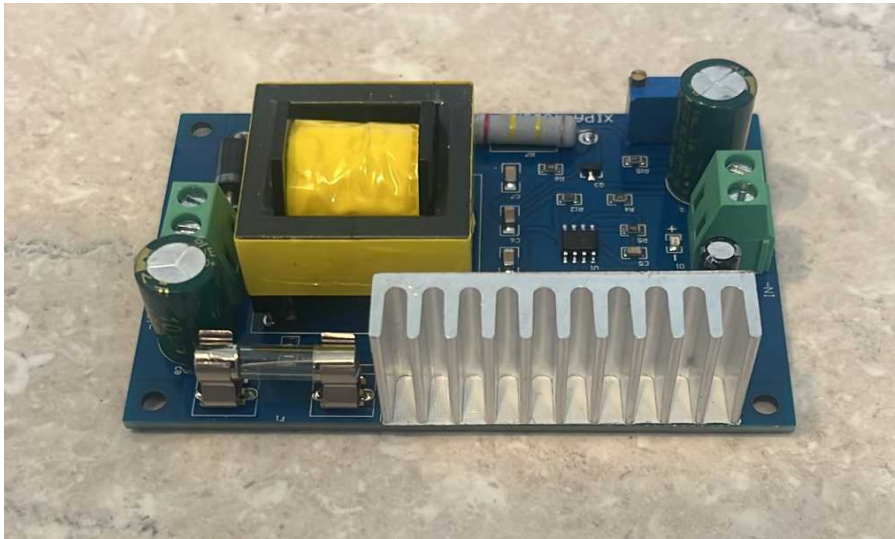
DC-DC Booster 12-24VDC → 160-400VDC 40W (XIPA-450CHV)
