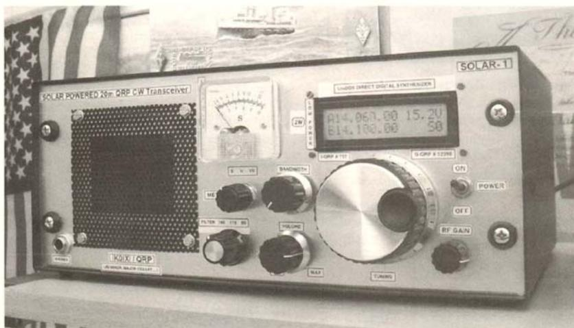
IK0IXI Solar Powered DDS Controlled 20m Transceiver
